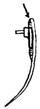
BRACKET SANDWICHED BETWEEN FUSELAGE AND FIBER MATT.
